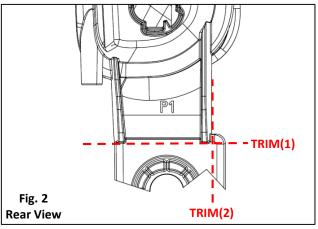
**2. Dry-Fit:** Dry-fit the repair tab(s) **Fig. 3**. If the tab fits without resistance and makes a flush fit to the housing, trimming is complete. If the tab resists installation re-trim the damaged tab, removing only small amounts of material. Repeat the Dry-Fit steps until the proper fit is achieved.
