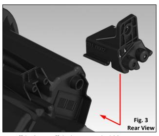
**3. Scuff & Glue:** Scuff the housing and tab(s) using a sanding pad. Remove sanding dust using compressed air. Wipe down the housing and tab(s) using a pre-cleaner to ensure surfaces are free from oil and debris. Apply glue to both the housing and tab(s).
